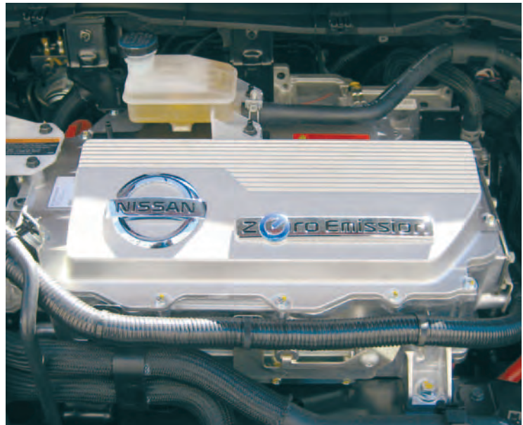
Under the hood of a Nissan Leaf. An EV contains no ICE; instead, the battery supplies electricity to the electric motor. Photo from Margaret Smith, DOE, NREL/PIX 18215
