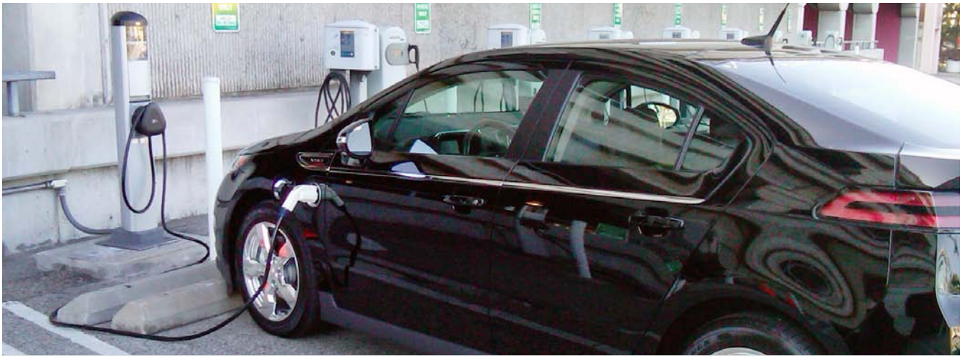
Figure 1. A Chevy Volt charges up with public Level 2 EVSE at Los Angeles International Airport. Photo from Coulomb Technologies
